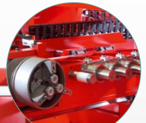
Tool magazine with forming tools and rotary forming unit
